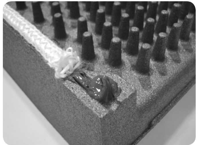
Figure 4b Placing of new silicone in the sockets.
